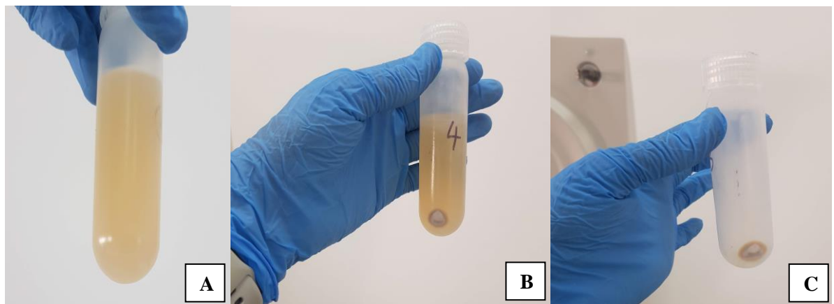
Figure 3.6 – Sediment after high-speed centrifugation of the supernatant obtained after the first low-speed centrifugation.
